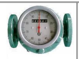
LC Series oval gear flow meter is developed based on market needs. It's immunity to the most viscous of fluids, oval gear meter are ideally suited for measurement of viscous fluids or those with varying viscosities such as oils, syrups and fuels. Ease of installation is another advantage of the oval design. Because no straight pipe runs or flow conditioning are required, oval gear meters can be installed in tight areas where alternate technologies would fail.
